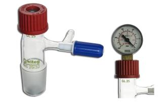
With function stop, with lateral 3 mm PTFE-valve, with screw thread, matching screw threaded necks.
