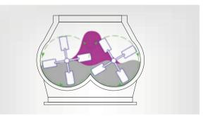
At this weightless zone, mixing of materials of different density is easy and fast because material particle can move freely and randomly, regardless of particle size and density. This brings a rapid and highly homogeneous mixing.
